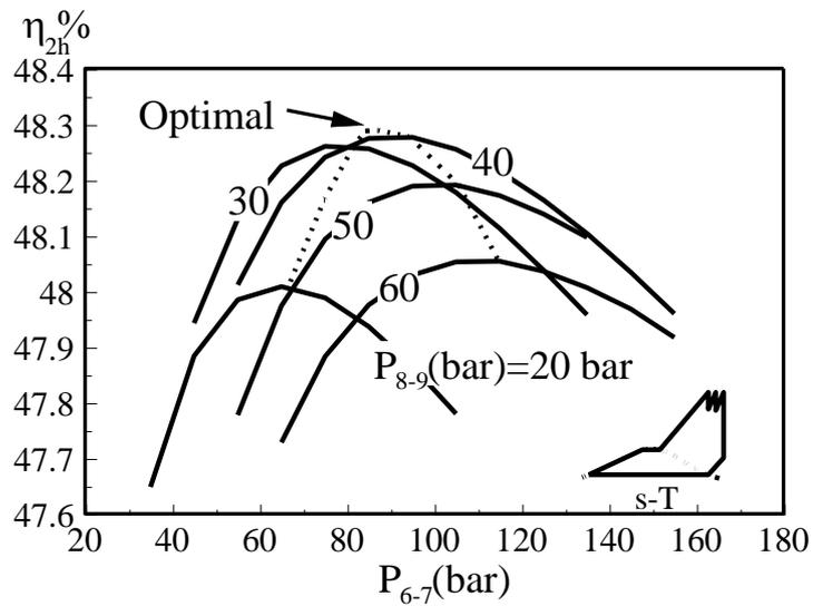
Figure 9: Effect of Intermediate Boiler Pressures,  $P_{8-9}$  and  $P_{6-7}$ , on TE of two-Reheating Stages RC
