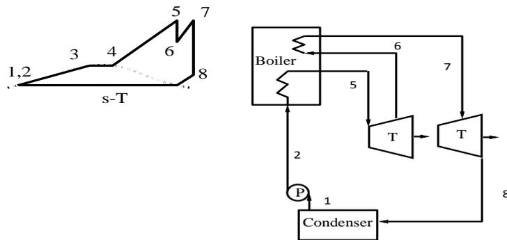
**Figure 2: RC with one- Reheating Stage**
