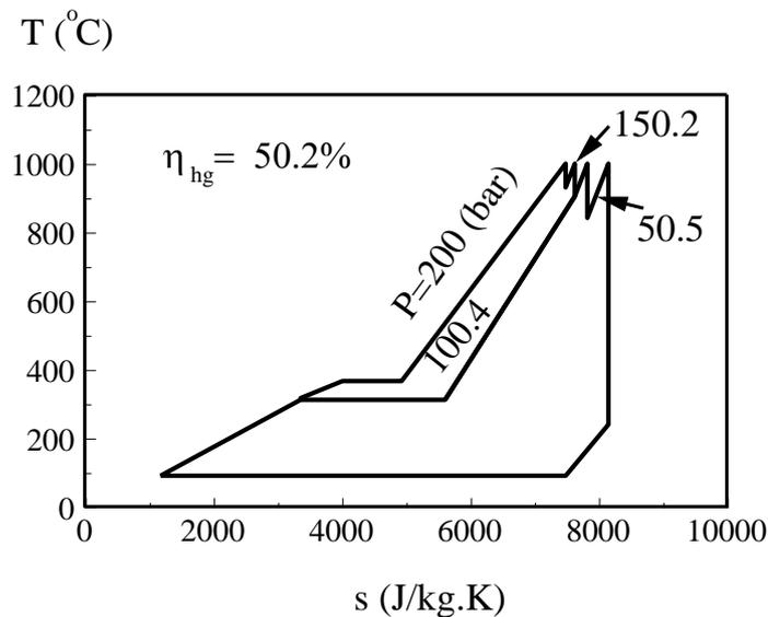
Figure 13: Thermal Performance of one-Reheating-one-Regenerative Stage RC with Equal Pressure Drops
