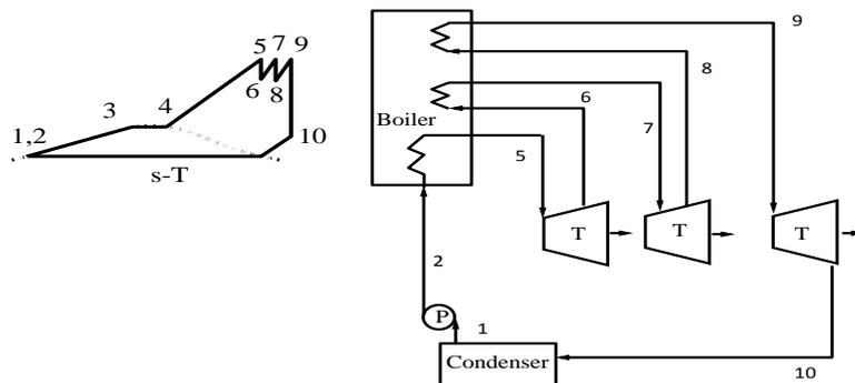
**Figure 3: RC with two- Reheating Stages**
