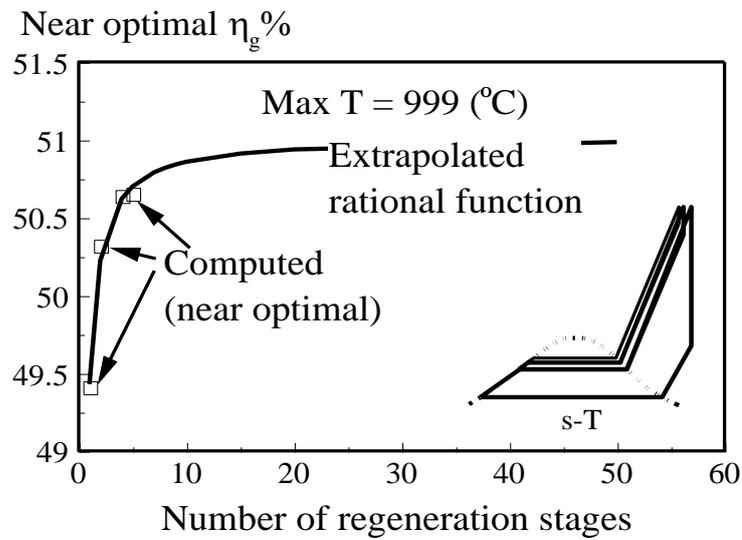
Figure 12: Effect of Number of Regenerative Stages on TE of RC
