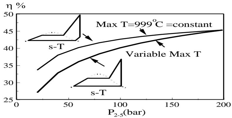
Figure 6: Effect of Boiler Pressure,  $P_{2,5}$ , and Superheated Steam Temperature on TE of Basic RC
