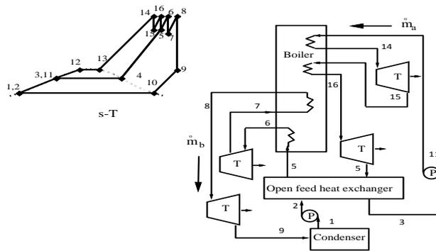
Figure 5 RC with one- Regenerative-one-Reheating Stage
