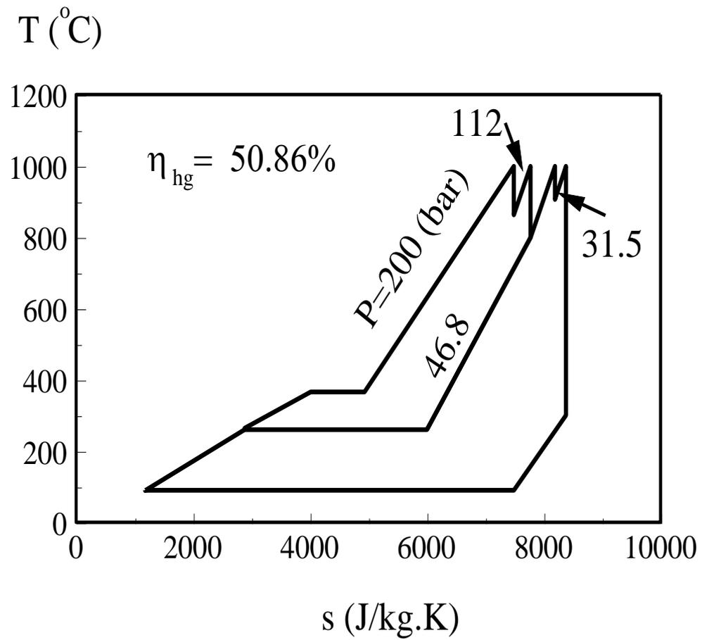
Figure 14 Thermal Performance of one-Reheating-one-Regenerative Stage RC with Non-Equal Pressure Drops
