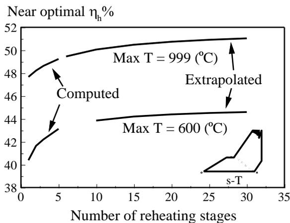
Figure 10: Effect of Number of Reheating Stages on TE of RC
