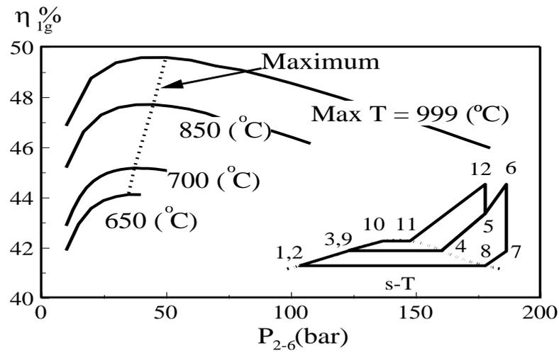
Figure 11: Effect of Intermediate Boiler Pressure,  $P_{2,6}$ , on TE of one-Regenerative Stage RC
