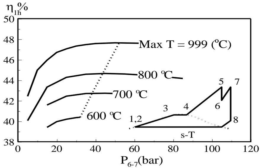
Figure 8: Effect of Intermediate Boiler Pressure,  $P_{6-7}$ , and the Maximum Cycle Temperature on TE of one-Reheating Stage RC
